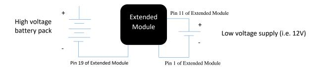
Figure 4 – Isolation resistance connection circuit
